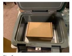
**Step 3.** Place one glycol USB Probe Data Logger that has been chilled to approximately 40°F inside of a cardboard box.
